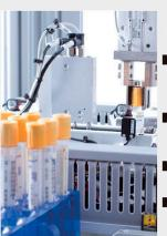
The test tubes are arranged standing and automatically inserted into racks
